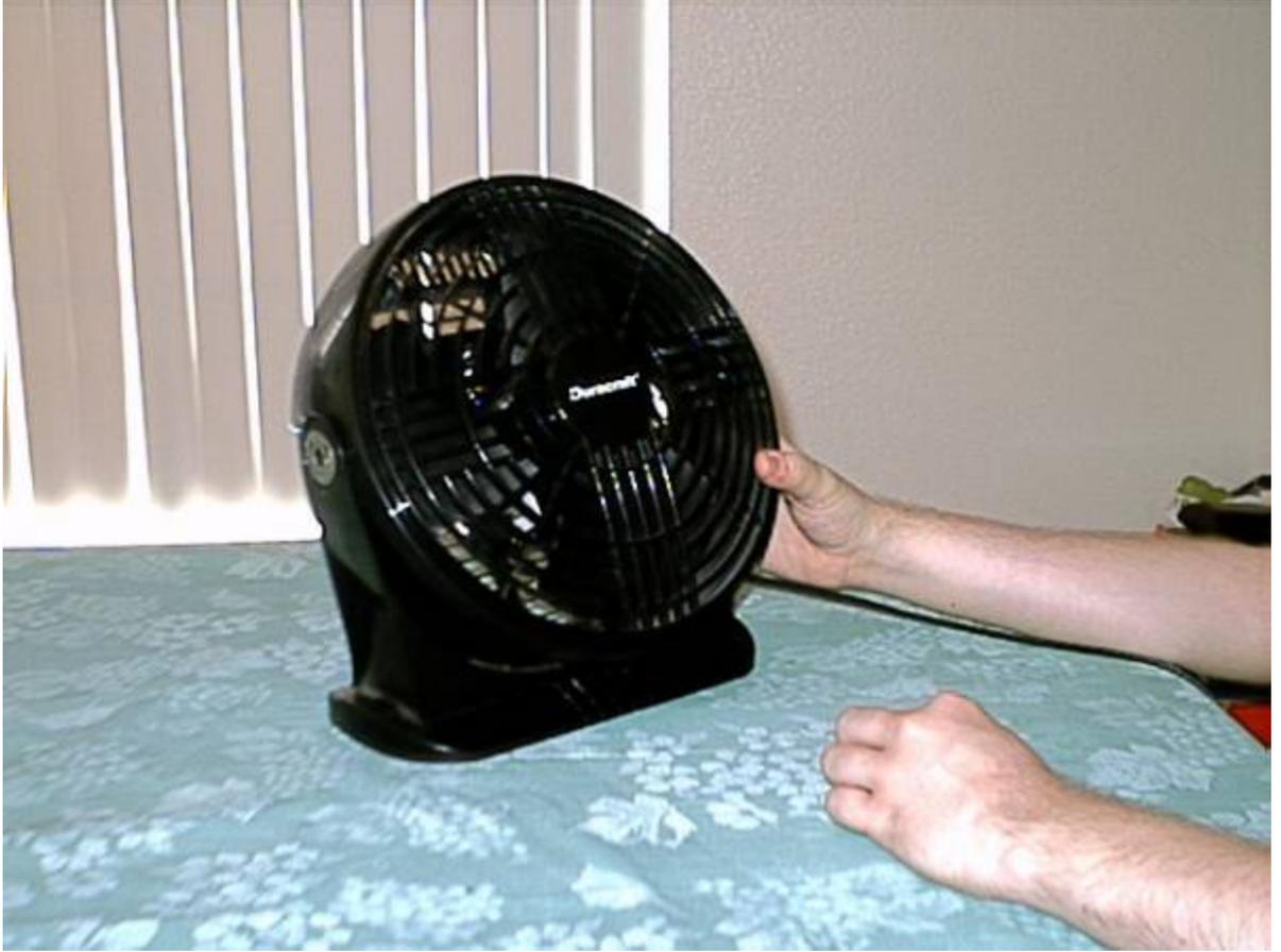
**Step 1:** Using a flat screwdriver, pry off the nubs on the base and remove the screws.
