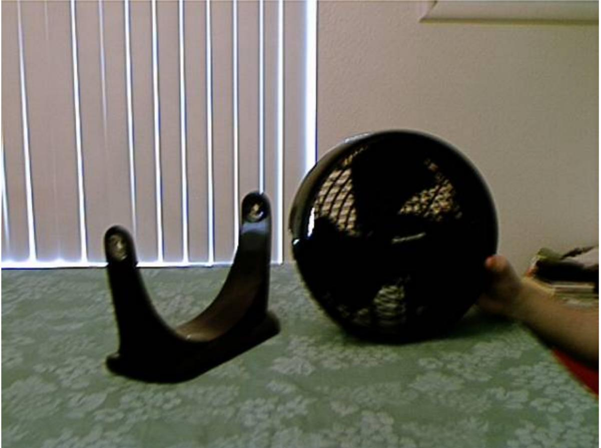
**Step 3:** Place the fan into the five gallon bucket, front side up. If you bought the Holmes brand fan pictured here it will fit VERY snugly. You don't even have to secure it in place.
