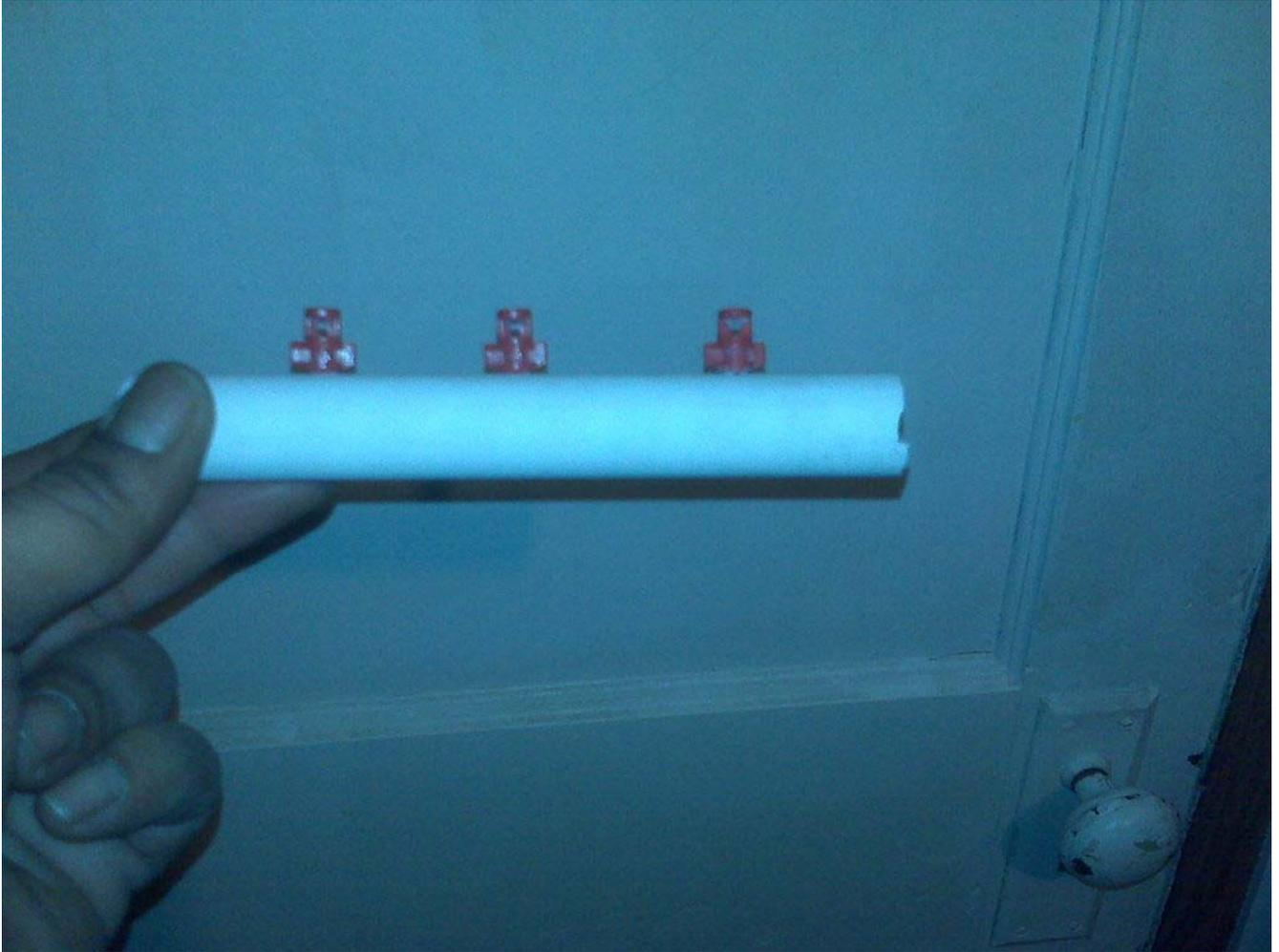
Now connect the pipes using the 3-hole 6" pipes for the outer frame, and the 2-hole 6" pipes with the 2.5" pipes to construct the center. I did not glue mine for various reasons, one being easy cleaning by total disassembly. Also, I want to be able to make slight adjustments if needed.
